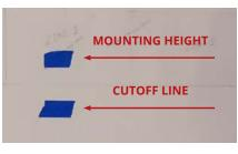
8. On your vehicle, measure the distance between the ground and the center of your SS3 pod. This is your mounting height.
