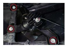
3. Install your assembled bracket and pod onto the vehicle by securing the three OEM bolts with a 10mm socket and ratchet.
