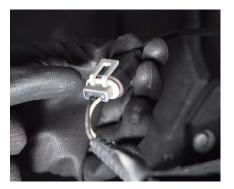
4. Plug the SS3 into the factory fog light harness using the included DT wire adapter. Test function. If the light does not turn on, try flipping the connector 180°.
