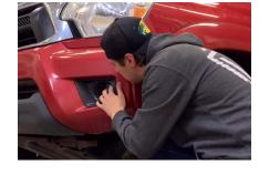
7. Loosen the 5/32" allen bolts on each side of your SS3 pod, just enough to allow you to adjust the pod.
