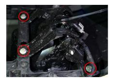
2. Access your factory fog lights and unplug the fog lamp connector. Use a 10mm socket and ratchet to remove the three bolts, as shown in the picture to the left. Remove the factory fog light housing. The factory bolts will be reused.
